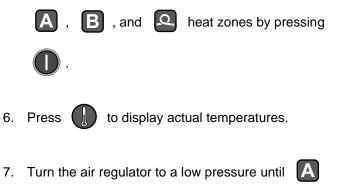
and **B** temperatures reach targets. Increase the pressure once the temperatures are on target.
