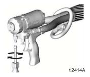
17. Disengage gun piston safety lock.
