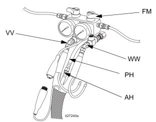
**NOTE:** Manifold hose fittings (VV, WW) allow use of 1/4 in. and 3/8 in. ID Reactor heated fluid hoses.
