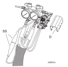
Connect cables (SS). Connect electrical connectors (NN). Be sure cables have slack when hose bends. Wrap cable and electrical connections with electrical tape.
