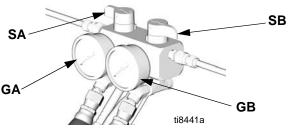
Check fluid pressure gauges (GA, GB) to ensure proper pressure balance. If imbalanced, reduce pressure of higher component by slightly turning PRESSURE RELIEF/SPRAY valve for that component toward PRESSURE RELIEF/CIRCULATION, until gauges show balanced pressures.
